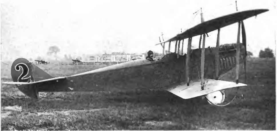
An aeroplane of the "tractor" type, so called because the propeller is attached to the front, pulling the machine through the air
