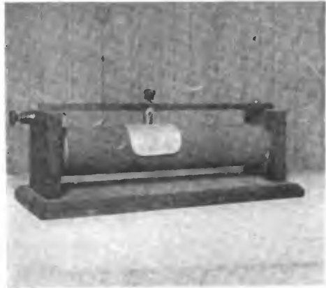
A photograph of the tuning coil used in the experiments described in the second prize article.
