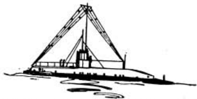
Detail view of aerial construction on the British submarine shown on the preceding page
