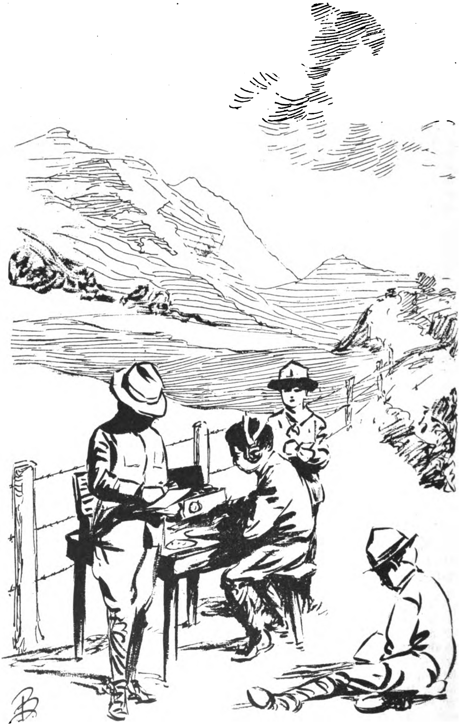
The barbed wire fence can be used as an aerial
