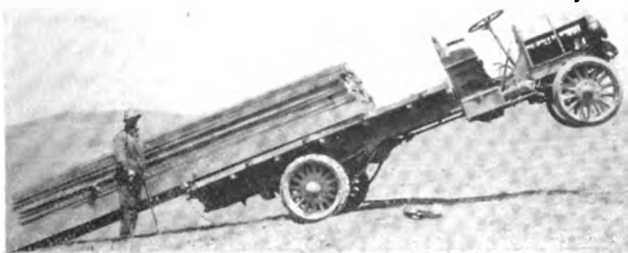
A bucking auto of the West; the result of leaving the overhang out of load calculations.
