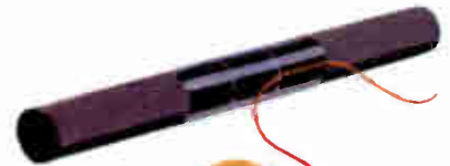
1 Wind the sticky tape in slightly overlapping parallel bands
