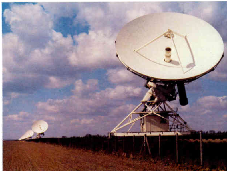
A radio telescope need not be a single dish-shaped aerial: it can be a whole set of aerials which together make a single receiver of radio waves from outer space. At the Mullard Radio Astronomy Observatory at Cambridge, this set of
