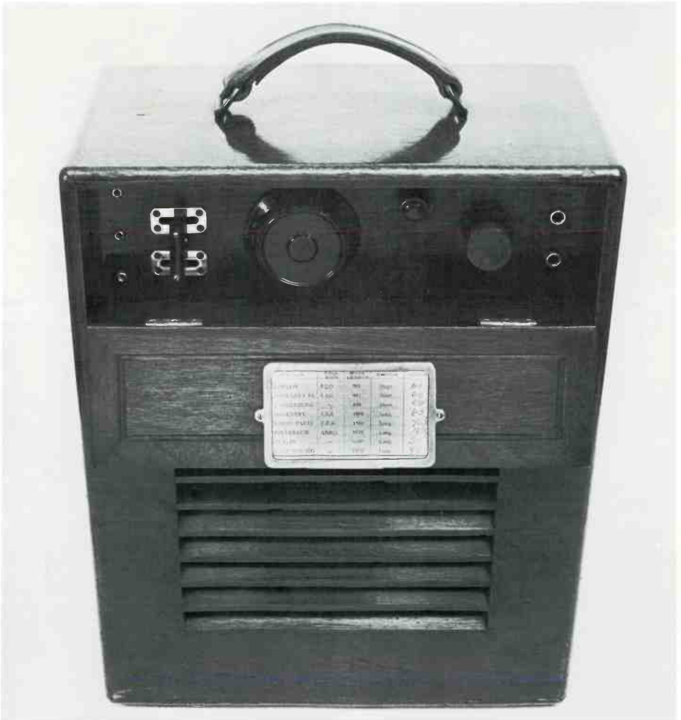
B4 Halcyon five-valve portable, 1927. Price: £33 1s (£33.05). Mahogany case with drop-down door revealing the control panel.
