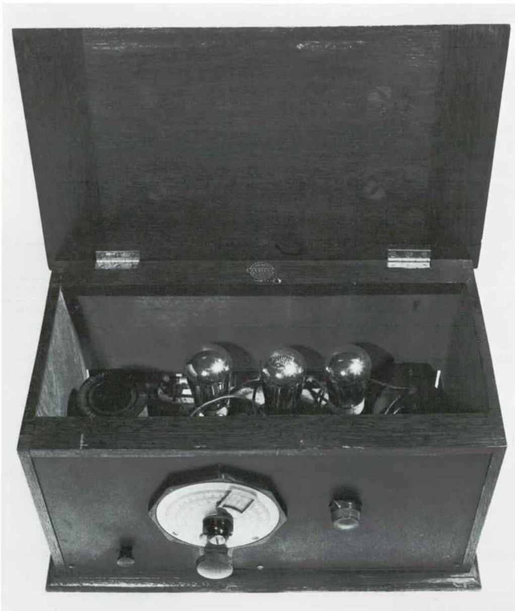
86 Three-valve home-made set in 'Hablok' cabinet, c. 1927.
