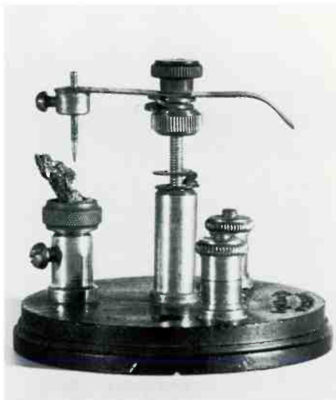
14 Detector by the Wainwright Manufacturing Company Ltd., c. 1920. The cat's whisker is in fact a steel needle fastened to a flexible brass strip, and is adjusted by turning the screw terminal in the middle of the strip.
