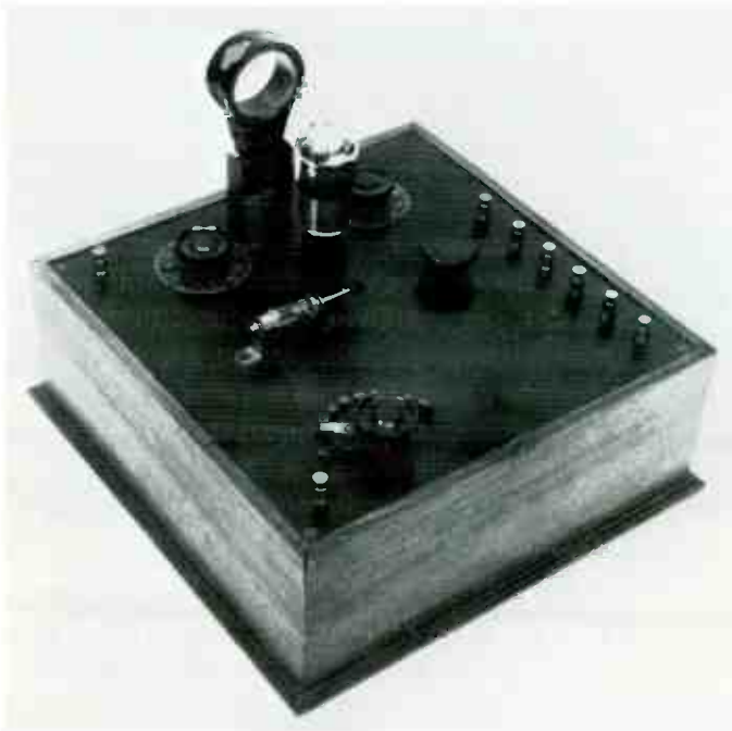
59 Combined crystal and single valve receiver. Home-made, c. 1922.
