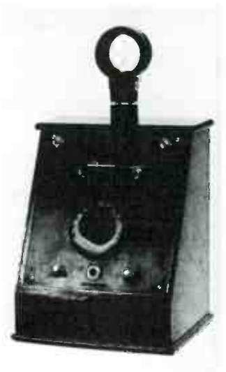
48 Home-made crystal set, c. 1923. Constructors could buy the cabinets ready-made and simply build their sets into them.
