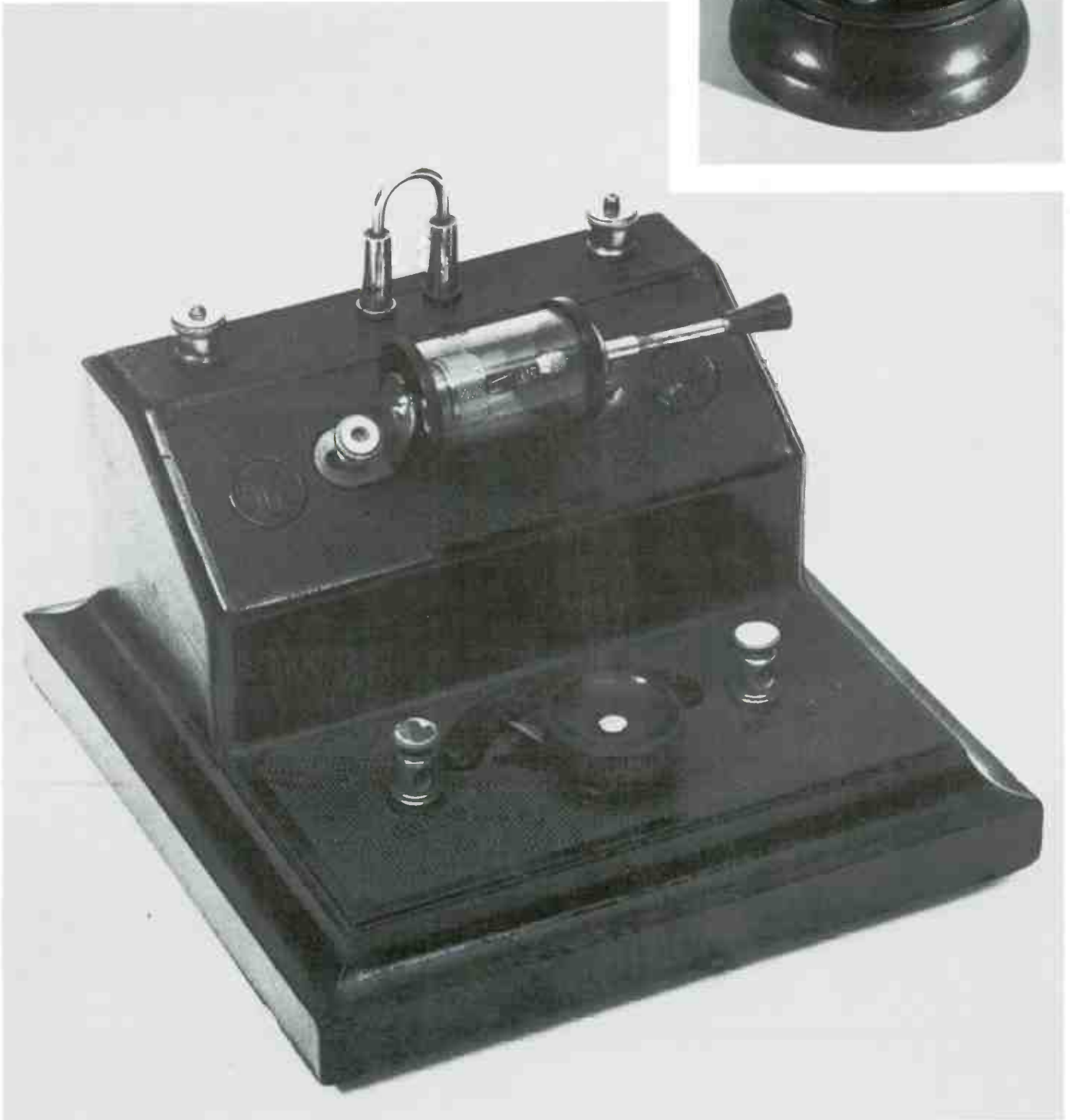
44 Brownie No. 2 crystal set, 1925. Moulded ebonite body. Price 10s 6d (52½p).
