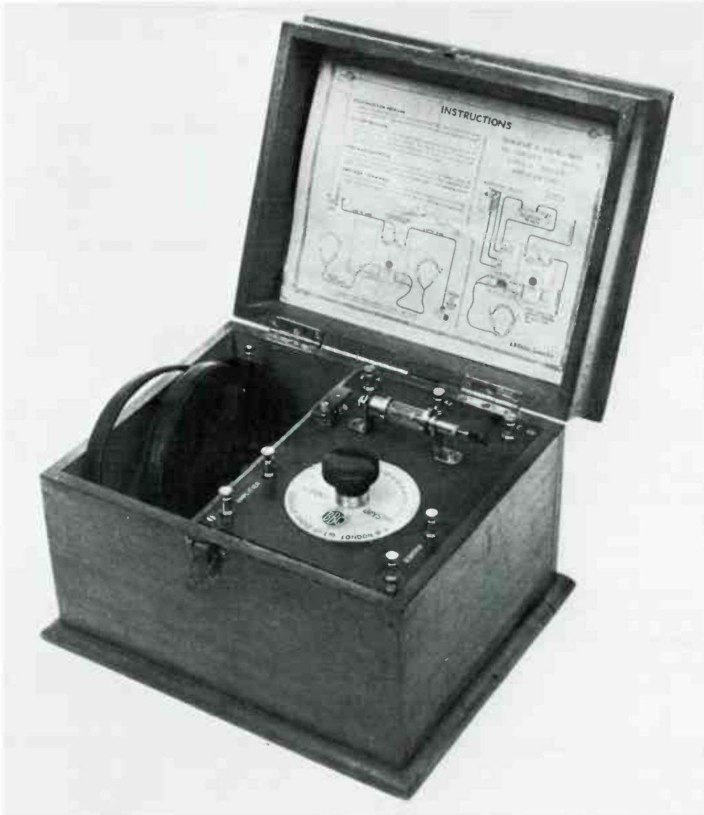
47 Crystal set manufactured by the Service Radio Company, 67 Church Street, Stoke Newington, London N.16, in 1924. Provision is made in the compartment next to the panel for connecting a Service one-valve amplifier which would give the listener greater station selection. Price of the set: £1 10s (£1.50).
