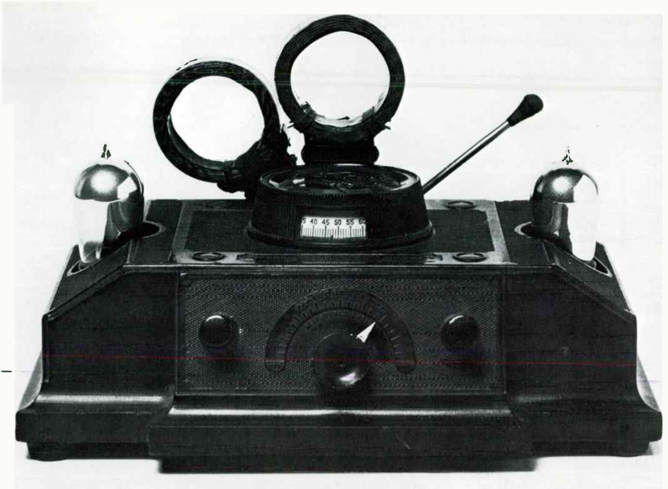
54 Brownie two-valve battery receiver, 1926. It used a loose coupled circuit operating up to 2000 metres and has plug-in coils. Moulded ebonite body. Price: £2 10s (£2.50).
