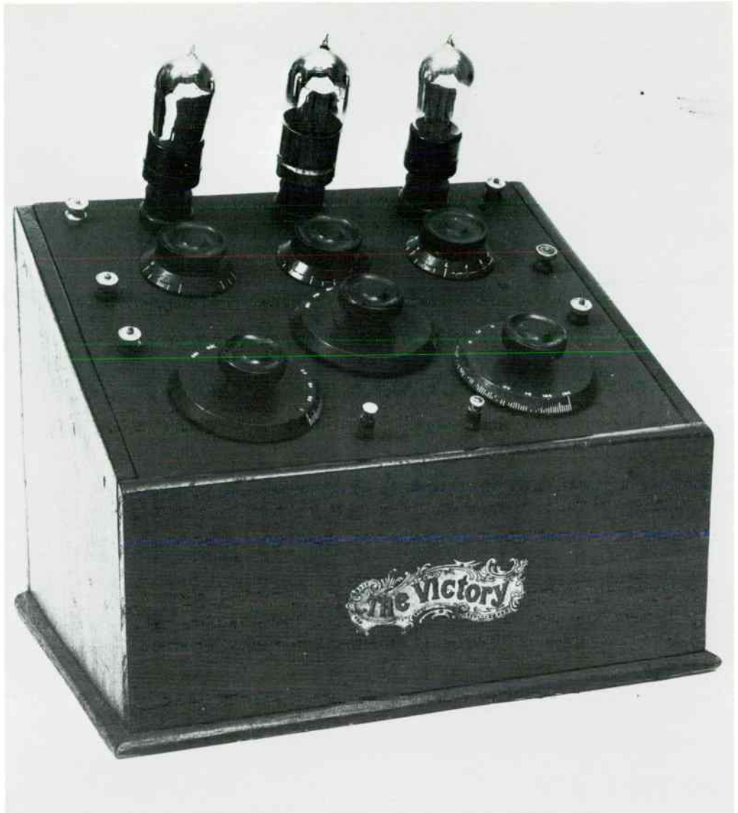
51 Victory three-valve sloping panel type receiver, c. 1922.
