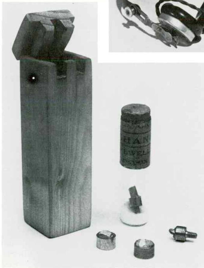
40 Elwell crystals. There are four different kinds of crystals housed in the glass tube, and these can be used in place of the Tellite crystal in the Elwell No. 11 set (ill. 39).
