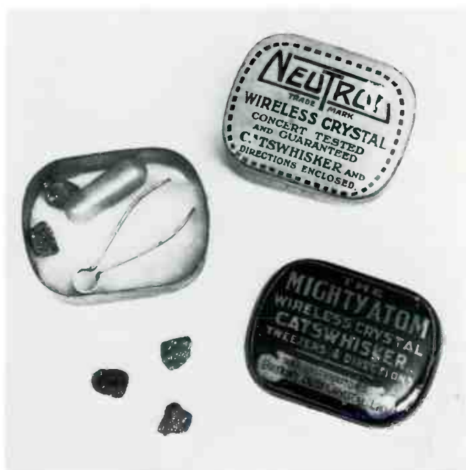
12 Mighty Atom and Neutron wireless crystals and cat's whiskers. In tin boxes complete with tweezers and instructions. Mid-1920s.
