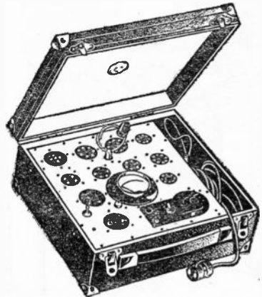
Fig. 13. A neat portable valve-tester (Norman Rose) which when operating draws from the mains.
