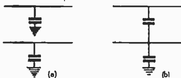
Fig. 13. Two ways condensers can be connected to by-pass asymmetrical currents to ground.
