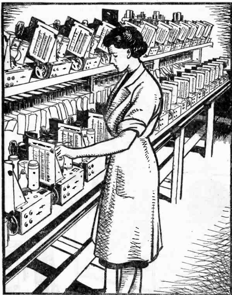
Fig. 13. Girls are employed a great deal in assembly work and increasing numbers are being used on repair and inspection. This girl is checking over a batch of completed chassis prior to fitting them into cabinets.
