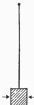
Fig. 7 (right) shows a simple illustration of inertia. A series of rapid blows on the sides of a heavy weight will not produce any movement.
