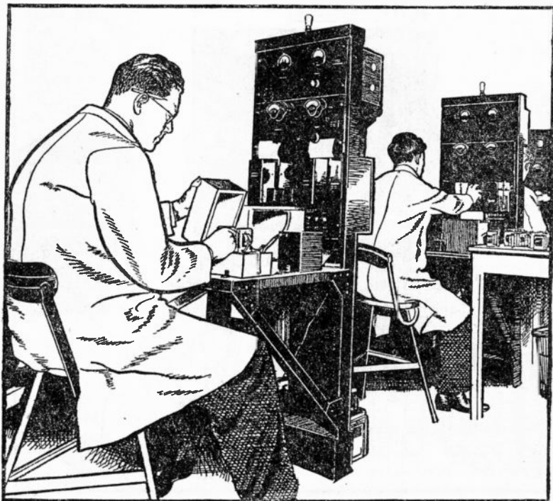
Fig. 21. Intervale and output transformers being checked against standards at several points on the audio-frequency scale.
