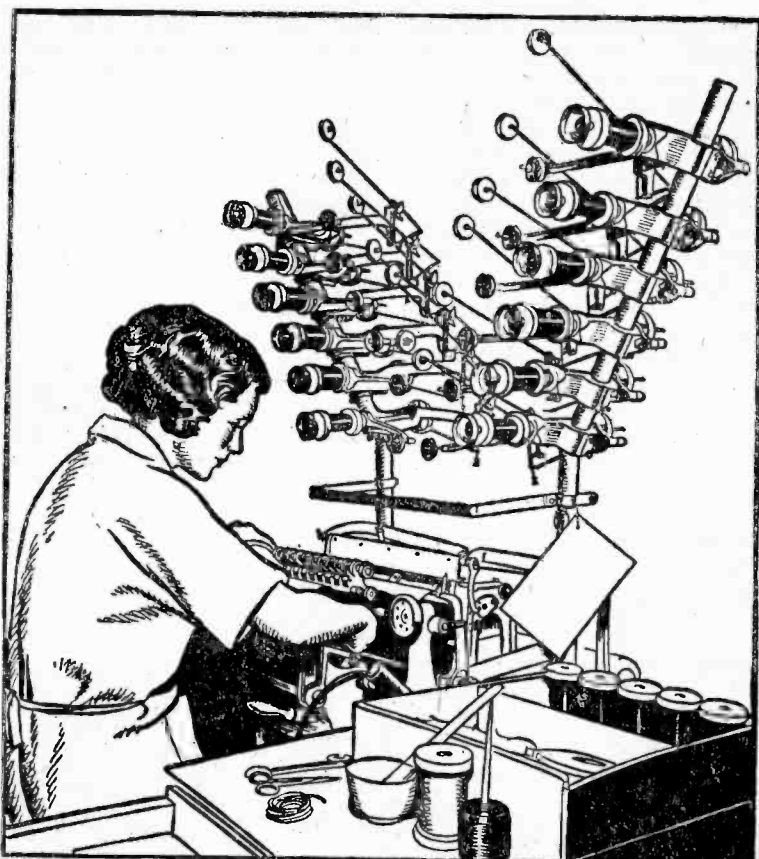
Fig. 18. A multiple machine, winding twelve coils simultaneously. The small rotating circular knives cut through the long former, thus making the individual coils.
