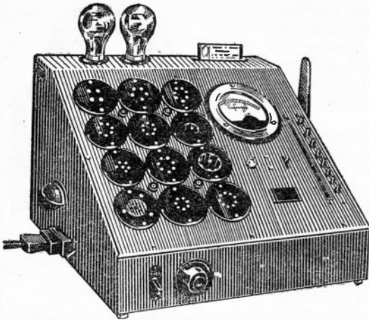
Fig. 12. The Mullard valve-tester. The valve is inserted in a holder, a special card is inserted at the top and all the necessary test connections are made either by pulling the lever or by pressing the buttons.
