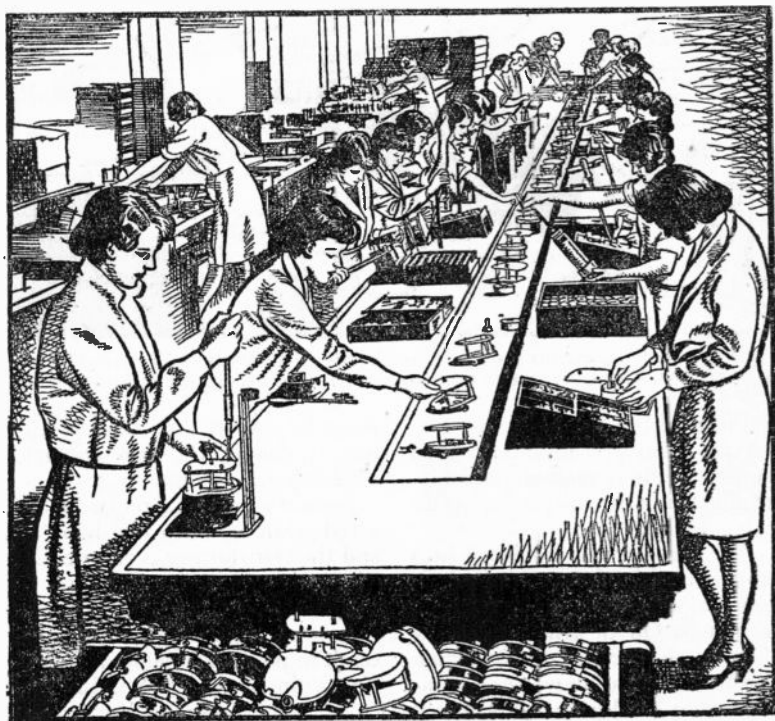
Fig. 17. Major components are assembled on a "line" as are receiver chassis. These girls are making up spring motors for portable gramophones and PA gear.
