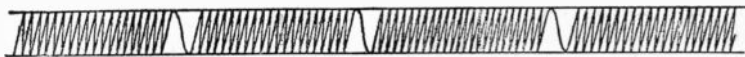
Fig. 31. Valve grids are wound in continuous lengths on a lathe, the wire being spot welded to the two support wires at each turn.
