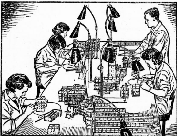
Fig. 4. Ganged condensers being mechanically inspected and their vanes adjusted.
