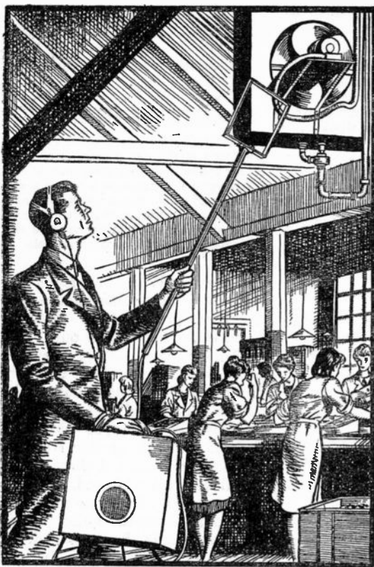
Fig. 10. The directional properties of a frame aerial can be used to locate interference-generating machines. An ordinary battery portable can be employed, but a separate aerial on a rod and headphones are of great assistance, particularly where, as in a factory, there may be a number of sources and considerable acoustic noise.
