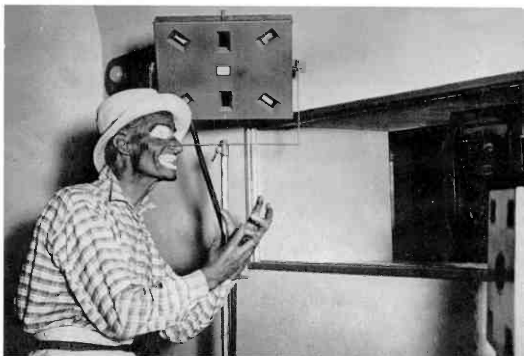
6f Fred Douglas in Studio BB at Broadcasting House, August 1936, as he appeared in the opening programme. Photocells (above and right), 'flying spot' came behind control-room glass (centre)
