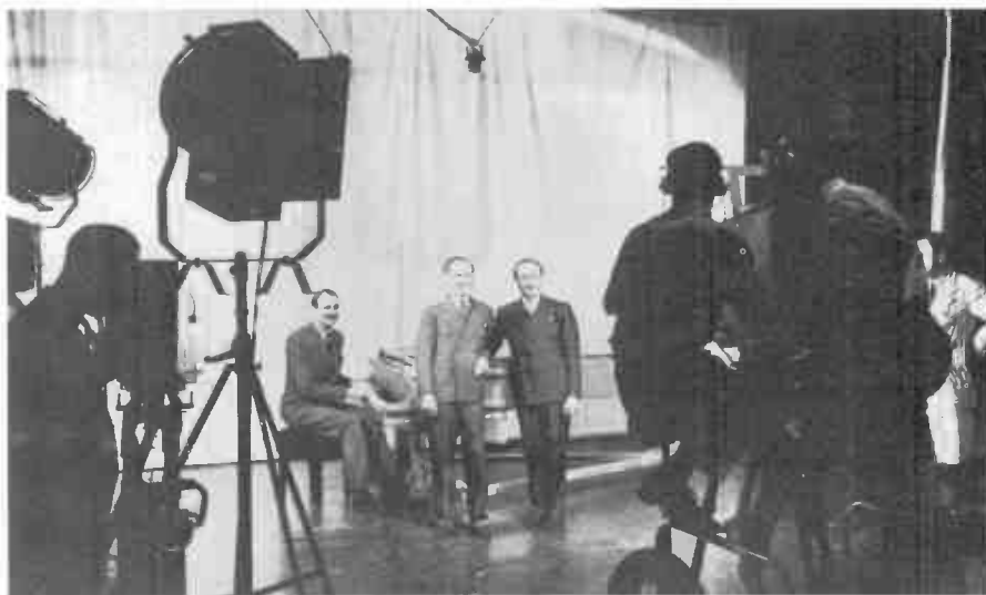
1c The Three Admirals. Stand lights and 'iron man' on left, camera on mobile 'dolly' on right. Headphone kept studio technicians in contact with the director in the control room
