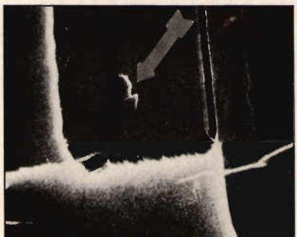
Fig. 3: SEM photomicrograph of a ruptured gate oxide.
