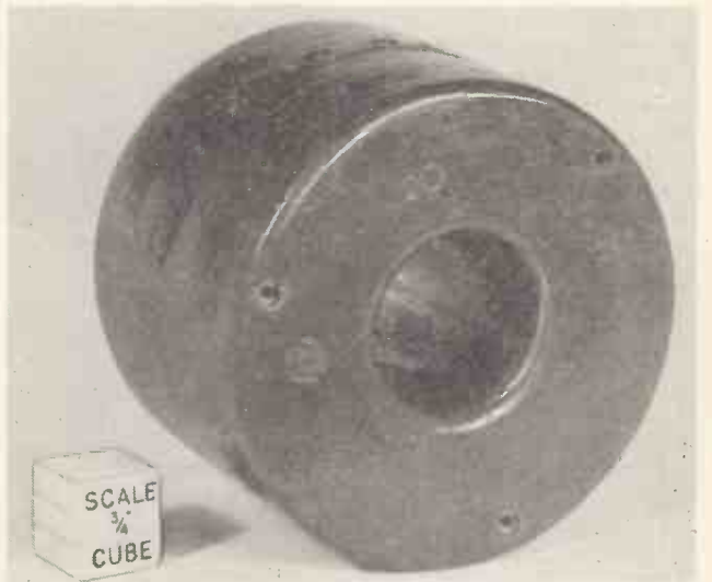
Fig. 3. The completed scanning-coil
