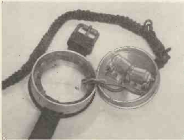
Fig. 2. Construction of the walking switch
