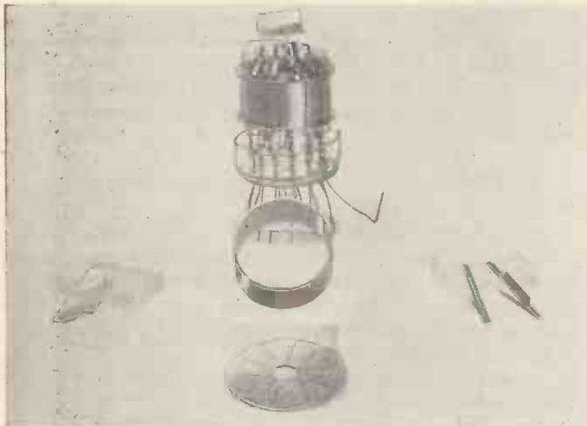
Fig. 15. Multi-gap valve and component parts
