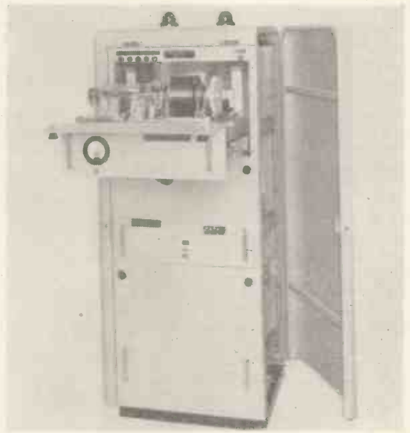
Cable & Wireless time division multiplex equipment.
