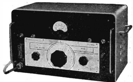
Beat Frequency Oscillator—AF200B —50 c/s to 20 kc/s—2 watts into 600 or 10 ohms—log scale to 1 kc/s.
