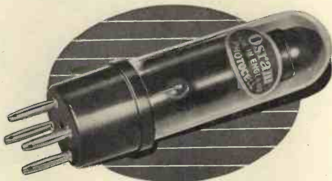
Dimensions: 92 mm seated length, 28 mm diameter and mounted on a four-pin British base.
