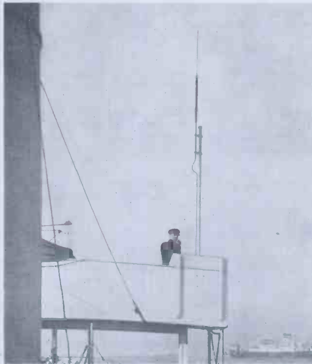
Fig. 6. Typical \frac{1}{2}\lambda aerial installed on ship's bridge
