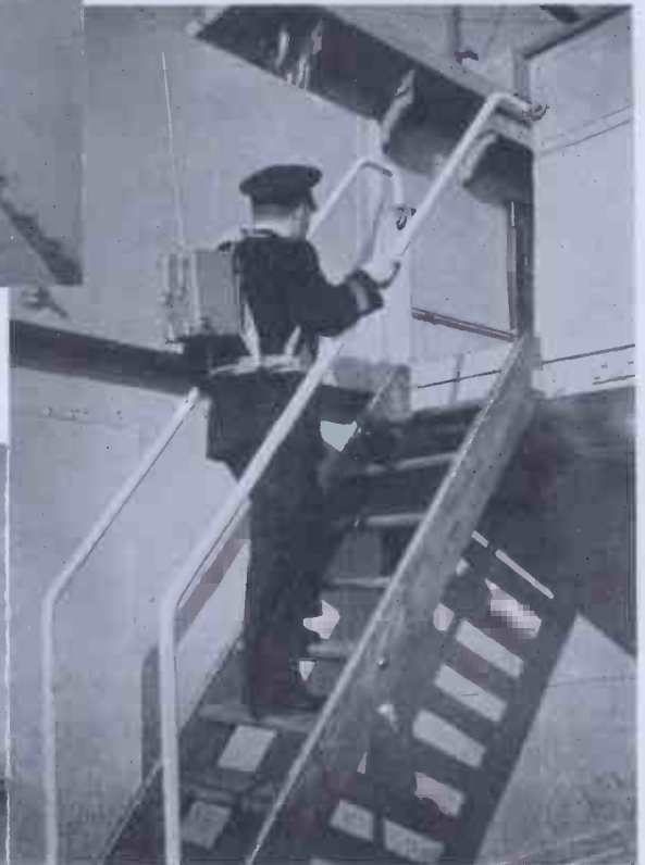
Locomotive driver using a Pye PTC 112/113 mobile Radio Telephone Set at a goods marshalling yard. The transmitter and receiver are housed in a special dust and fume proof protective case mounted just in front of the driver's cab. Power supplies are obtained from a steam driven 24V 500 c/s generator.
