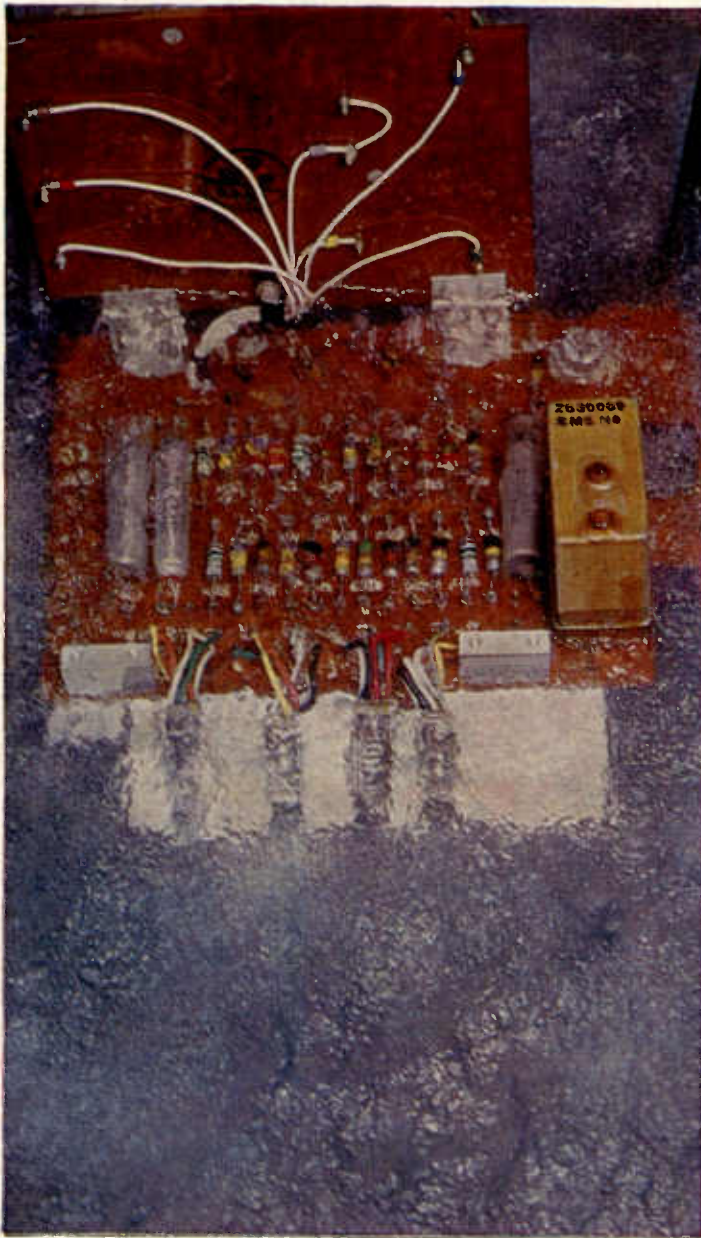
R.A.F. radar equipment being cleaned in 'Arklone' at the Ministry of Technology, Aeroplane and Armament Experimental Establishment, Boscombe Down. The cavitation effect of ultrasonic cleaning in the ICI plant is clearly seen.
