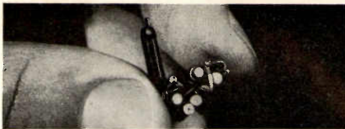
This prototype hearing aid amplifier, developed by SGS-Fairchild Applications Laboratories using the HA10 hearing aid package, delivers a power output of 0.4mW into a load of 1000Ω when operated from a 1.5V supply; battery drain is 2-1mA.
