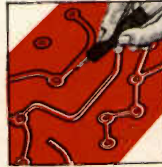
With sharp blade, outline the areas to be masked. Do not cut through the backing sheet. The Ulano Swivel Knife does the job quickly, easily.
