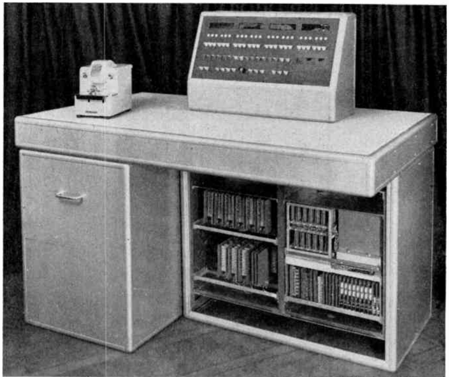
Fig. 7. Digital computer designed to incorporate microminiaturization techniques The nearest equivalent using conventional techniques occupies four standard 7ft racks, plus a control desk. The new computer is entirely contained within the control desk and is 10 times faster than the conventional versions
