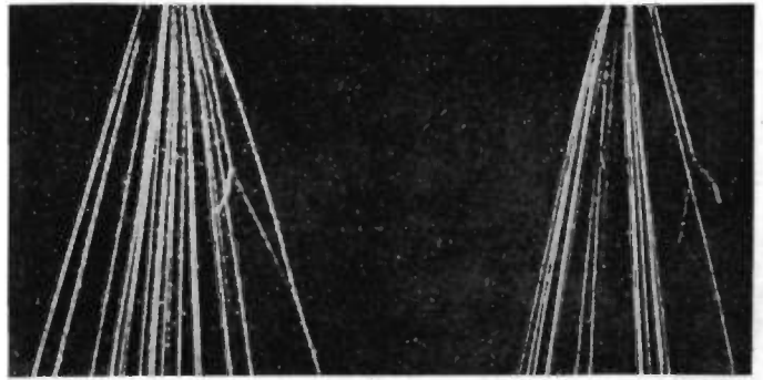
Fig. 8. Stereoscopic photographs showing \alpha -particle tracks in nitrogen. The forked track indicates an inelastic collision with a nitrogen nucleus resulting in the ejection of a proton. —"Radiations from Radioactive Substances" by Rutherford, Chadwick & Ellis, (Cambridge Press.)
