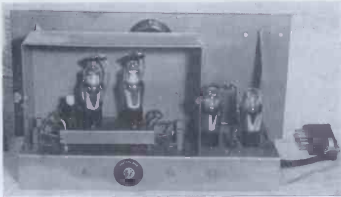
Fig. 1. Interior of aperiodic generator showing anti-microphonic mounting of sub-chassis.
