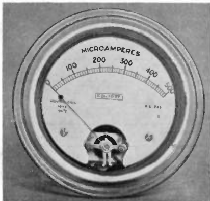
Fig. 3. Special glass-cased hermetically sealed meter for tropical use.
