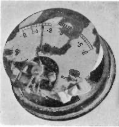
Fig. 2 (left). A standard commercial meter, after 6 weeks' tropical test. (Temperature 25°C.—40°C. continuous cycle. 95 per cent. Relative humidity.) Note the almost complete obliteration of the scale markings, and disintegration of pointer. The rest of the mechanism on this model is cadmium plated, and has stood up well to the test. Meters with a less satisfactory finish, corrode very badly.
