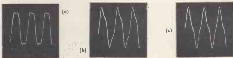
Fig. 9. Addition of fundamental and 3rd harmonic with different phase displacements due to time delay through the amplifier.
