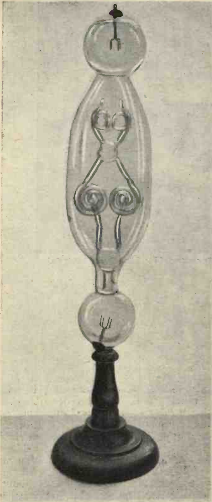
One of Geissler's ornamental discharge tubes.
