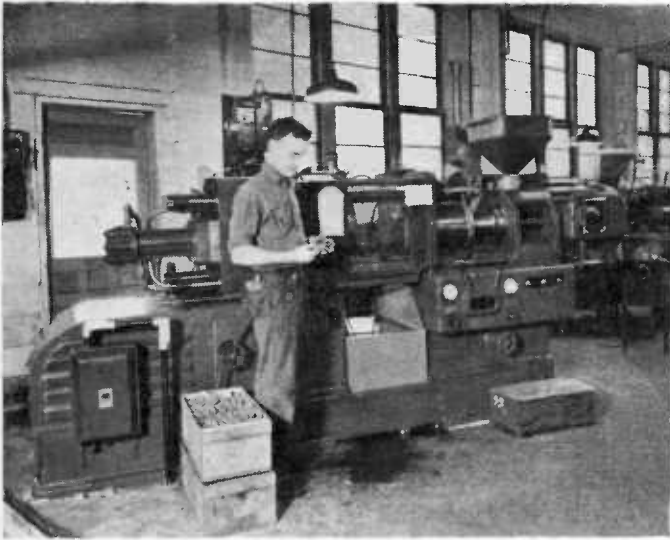
Fig. 1. Automatic machine for mass production of injection mouldings. The operator is holding a set of mouldings which have just been expressed from the machine.
