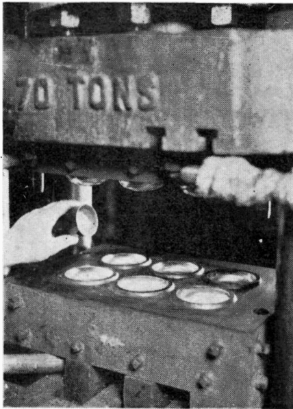
Fig. 7. Moulding of Bakelite (Loading mould). Courtesy of Bakelite, Ltd.
