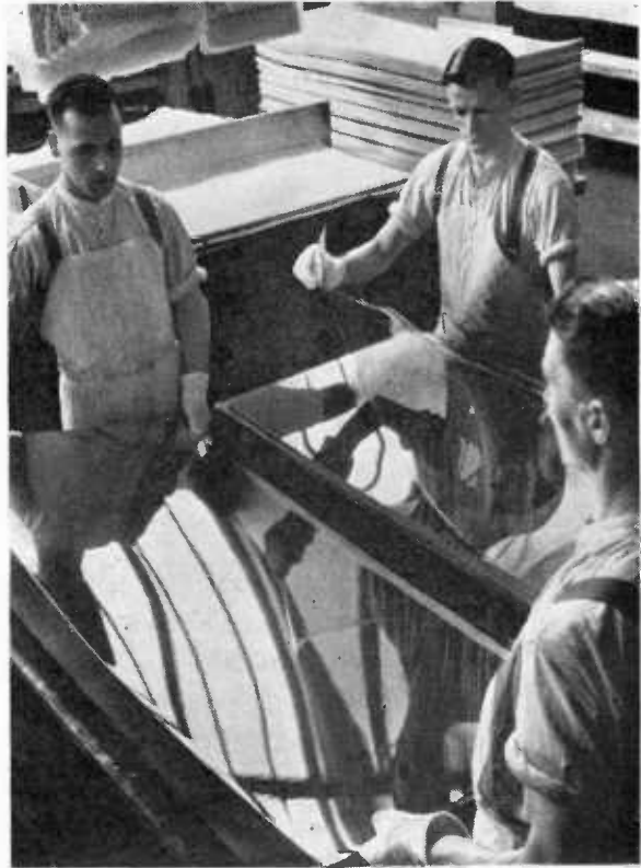
Fig. 2 (right). Removing polished celluloid sheet from polishing "nip." Courtesy of BX Plastics, Ltd.
