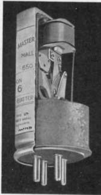
Fig. 1. Sectioned vibrator unit showing driving magnet, reed and contacts.
