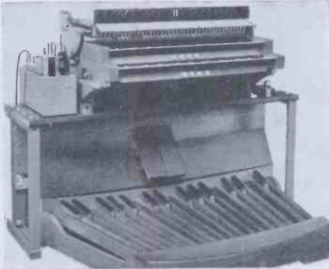
Electronic organ with case removed.
