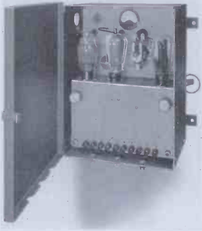
Fig. 6. Photo-electric relay for single-way register control.
