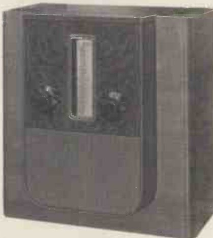
This is a new Murphy receiver which has been modified to cover the 160-metre amateur and commercial waveband.
