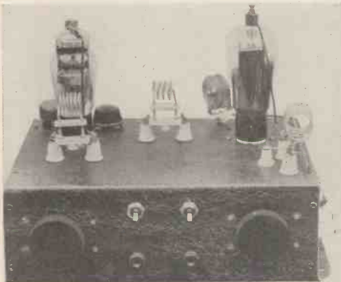
All the components are mounted on this small chassis. The coils are of the Eddystone interchangeable type so that the unit can be used on 10 and 5-metres as required. The P.A. valve, an E.S.W.20, provides a high carrier power on 5 metres.
