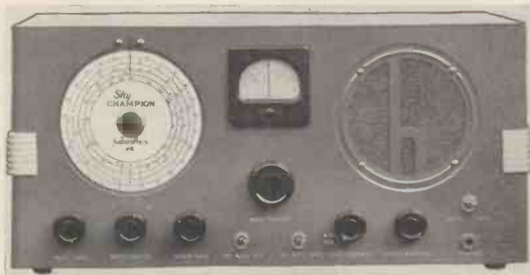
All the controls can be seen in this illustration. The band-spreading arrangements deserve special note.
