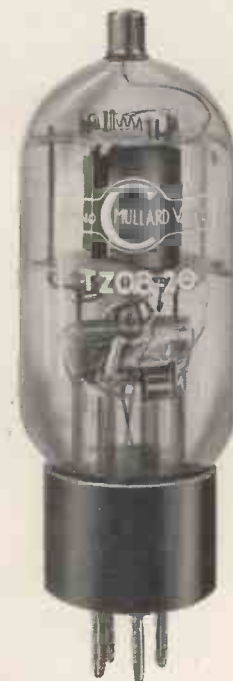
Mullard have provided this new triode for amateur service. It electrically replaces the T-20.
