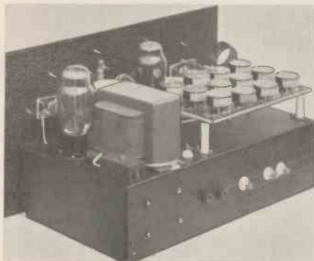
This view shows how the crystals are mounted on a sheet of Trolitul. In this way sockets can be used instead of the more normal crystal holders. The insulators are for link coupled or capacity coupled output.
