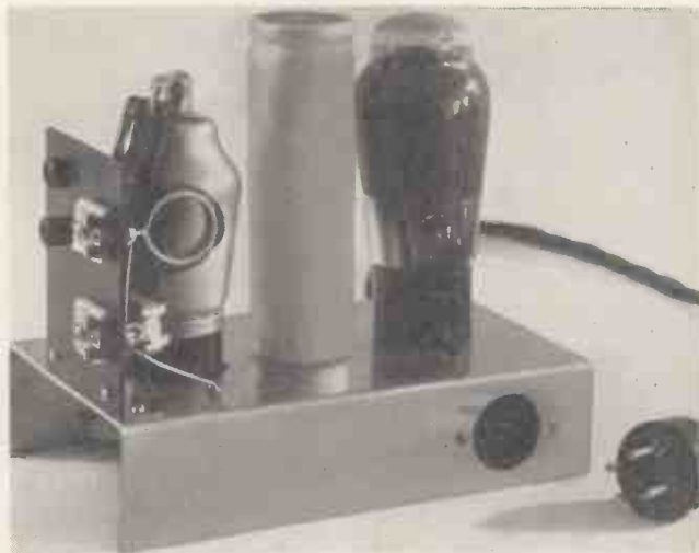
Tuning condensers are mounted directly on the miniature front panel. A separate power pack is needed and is connected by means of four-pin socket into the valve holder on the side of the chassis. Notice how the grid connections in the detector circuit are kept very short.
