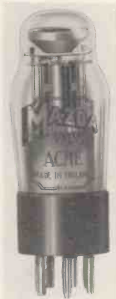
The AC/ME cathode-ray tuning indicator is fitted with a 7-pin base and designed for horizontal mounting.
