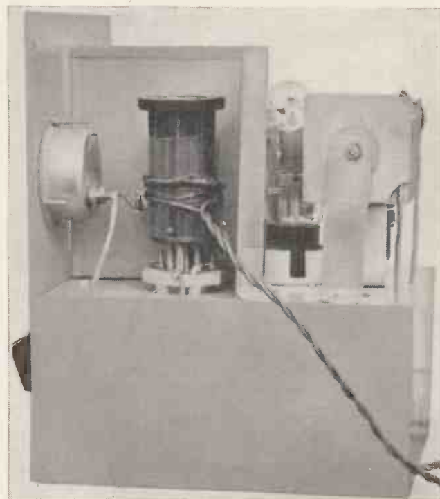
Link coupling to the transmitter is used and a coupling made by a flexible wire in the manner shown.
