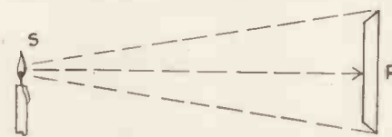
Fig. 1. Diagram showing how luminous intensity is determined.
