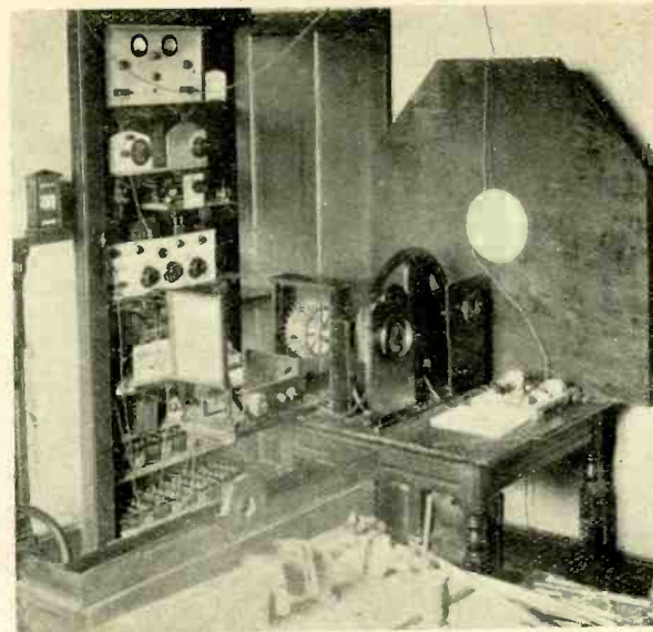
Notice the positioning of the front screen with reference to the mirror drum
