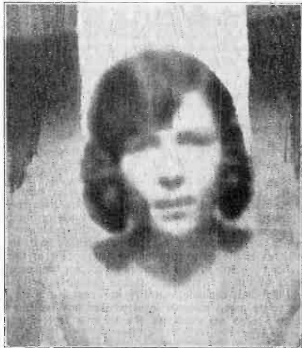
Illustration A.—Demonstrating the bad effects produced in a television image when there is a considerable loss of the lower frequencies.
