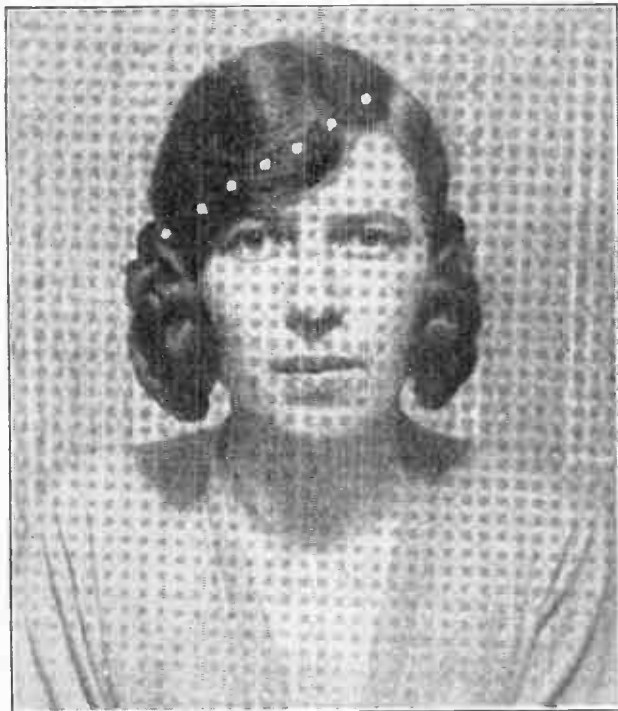
Illustration C.—Heterodyning takes the form of a fairly fine mesh over the whole of the image.
