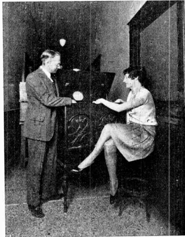
Photograph of Zworykin's new cathode-ray television receiver. The images are projected on to a mirror on the top of the cabinet, thus making it possible for a number of people to watch at once.
