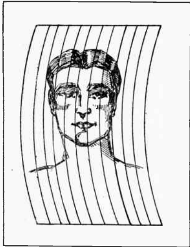
Fig. 2.—How a television image is built up of closely fitting strips.
