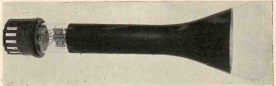
Fig. 7.—A modern high-vacuum tube with a 6-in screen (Standard Telephones and Cables).
