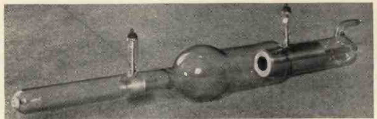
Fig. 2.—Perrin's tube which demonstrated the negative charge associated with the electron.
