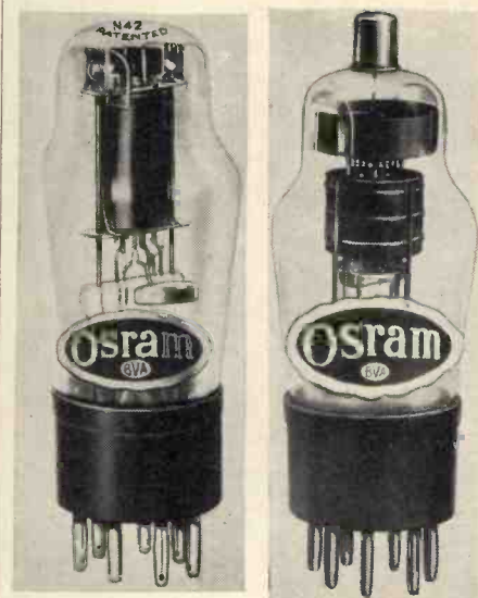
This is the N42 L.F. pentode with the W42 H.F. pentode on the right.
