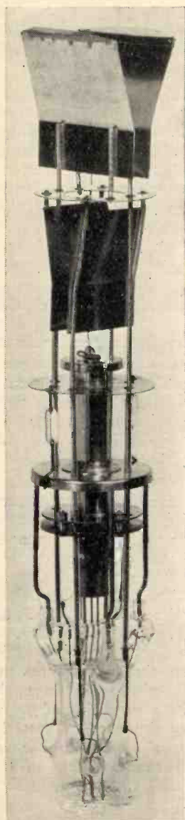
Fig. 1.—This is a photograph of the latest Ediswan cathode-ray tube electrode assembly. It is constructed as a complete unit before insertion in the neck of the glass bulb.
