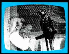
Co-channel interference. Signals from another transmitter operating on the same channel can give rise to the effects shown here. See *Umusual Atmospheric Conditions*
