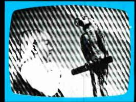
Local oscillator interference. This form of wavy patterning on UHF can be caused by a nearby television receiver tuned to a VHF station.
