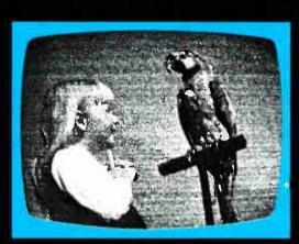
Weak Signal. Low signal strength, often resulting from an inadequate or poorly adjusted aerial, can result in a 'noisy' or grainy picture.
