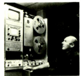
VTR machines enable pictures and sound to be recorded on tape and replayed on a monitor screen or for transmission. Granada
