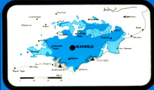
139 HEATHFIELD UHF Main Station Ch64 Relays: Hastings Ch28; Newhaven Ch43*
