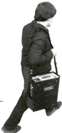
▶ A portable video tape recorder of the type currently in use for electronic news gathering. Already, the engineers are working towards integrating the recorder into the camera itself.
