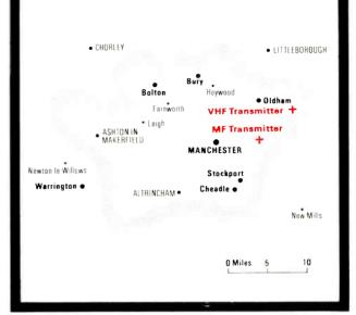
IBA Transmitters VHF Transmitter (FM with stereo capability) Saddleworth (NGR: SD 987 050) 97.0 MHz Max erp 2 kW Circular polarisation Aerial ht. 1278 ft aod
