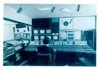
3. Sound is not the poor relation of television. This is the sound control suite of a modern studio where the levels from the many microphones are blended and balanced and effects added from audio tapes or discs.
