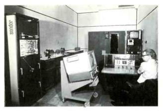
7. The telecine operator runs a film in the enclosed machine in the background to provide a television-signal output.
