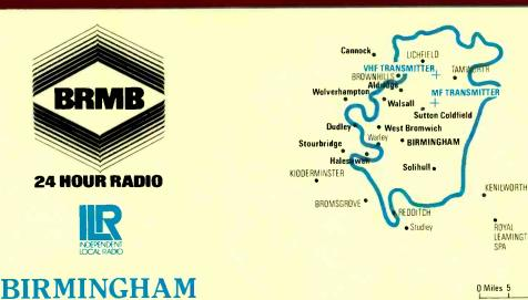
Circular polarisation Aerial ht. 1390 ft aod MF Transmitter (medium wave, mono only) Langley Mill (NGR: SP 160 968) 261 m (1152 kHz) Transmitter power 0.8 kW
