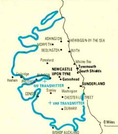
VHF Transmitter (FM with stereo capability) Burnhope (NGR: NZ 184 474) 97.0 MHz Max erp 5 kW Circular polarisation Aerial ht. 1 407 ft aod
