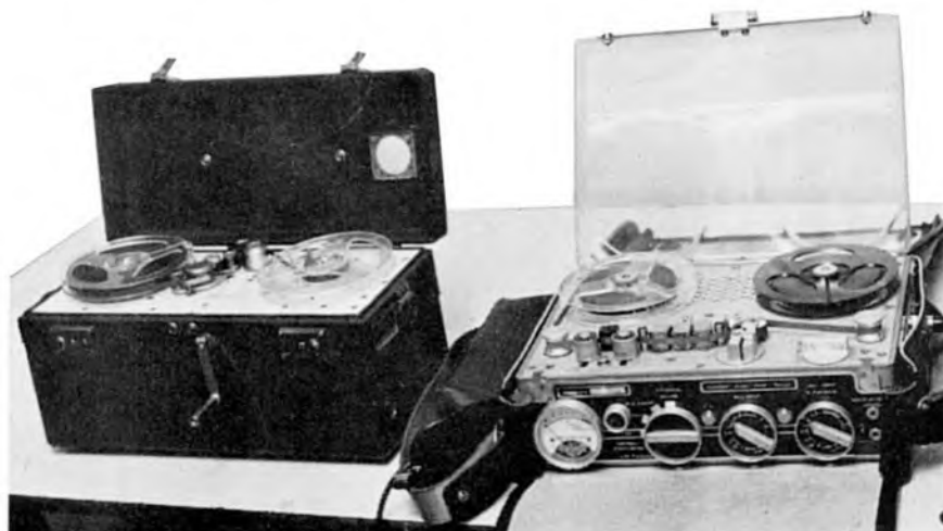
Two famous pieces of equipment stand side by side. On the left is the time-honoured Boosey & Hawkes battery portable with hand-wound clockwork transport system. Next to it the aristocratic Nagra, one of the most famous of all professional battery recorders. Truly an historic meeting!
