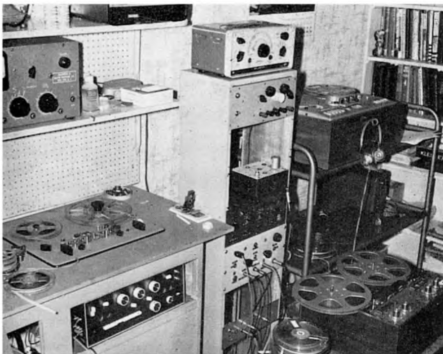
The author's studio for general recording, showing, left, Brenell deck for copying full-track or half-track with Rogers stereo amplifier below, centre, rack containing mixer, patching boards, small oscilloscope and on the right a Telefunken M24 full-track recorder with a Revox R77A half-track stereo machine below
