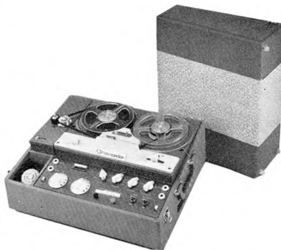
A general view of the Cinecorder, showing deck and controls and the detachable lid containing the speaker
