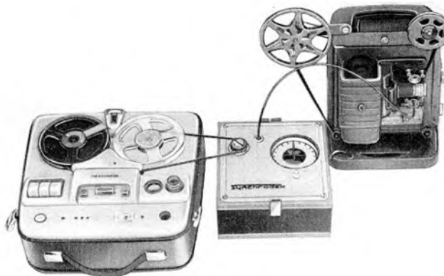
The Synchronode can be used with any recorder and variable-speed projector to indicate synchronism. It is here seen linking a Telefunken recorder and a Bell and Howard projector
