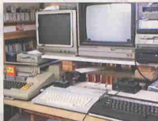
A selection of Atari 8-bits and accessories. The machine on the far right is a rare American 1200XL, never sold in the UK, and just above it can be seen an Indus GT disk drive with, above that, an 830 acoustic coupler!
