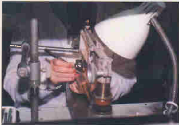
Winding of mesh filament for the Svetlana 3CX3000A7 and 4CX10,000D.
