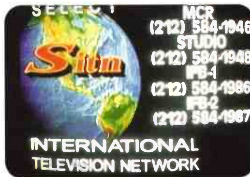
This New York facility regularly appears on both PAS-3R @ 43°W analogue and NSS-K 21.5° capacity (MCR = Master Control; IFB = Interrupted Fold Back - a keyed reverse studio sound guide for the remote reporter's ear piece).
