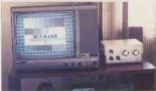
A relatively simple DX installation consisting of a standard TV receiver, a D-100 DXTV converter fed by an external antenna.
