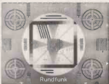
The German 'T05' monoscopic test card radiated in the Sixties and early Seventies by Hessischer Rundfunk.
