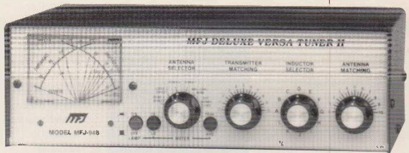
Fig. 7: Antenna tuning units: a) receiver only; b) Versatuner for both transmitter and receiver use.
