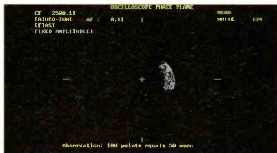
Fig. 7: One of the other unique features on a measuring tool of this cost is the 'Phase plane' module. Here is the plot of a p.s.k. (phase shift keyed) system. Note the activation of the 'Auto-Tune' facility, which is keeping the signal locked to counteract both transmitter and receiver drift. There isn't too much drift occurring in either here though as the Code30 is only having to correct by 0.11Hz.
