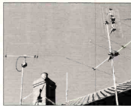
Fig. 5: A new antenna system under evaluation by Roger Bunney (Romsey). The antennas to the right (the u.h.f. grid and 4-element f.m.) are for domestic reception while the one on the left is a rotatable wideband Band I array for sporadic-E DXing.
