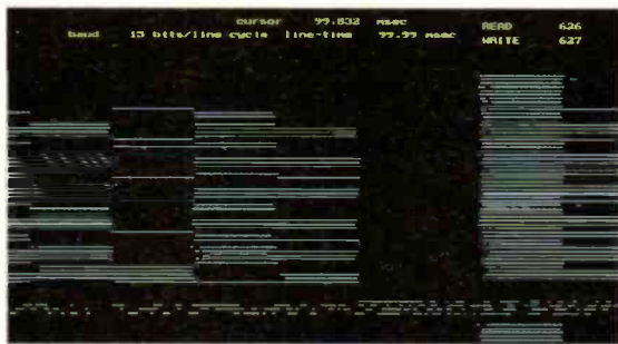
Fig. 5: The 'Speed-Bit Analysis' module allows the use of movable on screen cursors (not shown) to make timing measurements. Here the signal can be seen to have a consistent pattern with the same bit occurring in the right hand side of the display.
