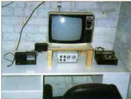
Shaun's shack showing his D-100 DXTV converter, portable TV and f.m. radio. The radio allows the various TV sound systems to be heard via the D-100.
