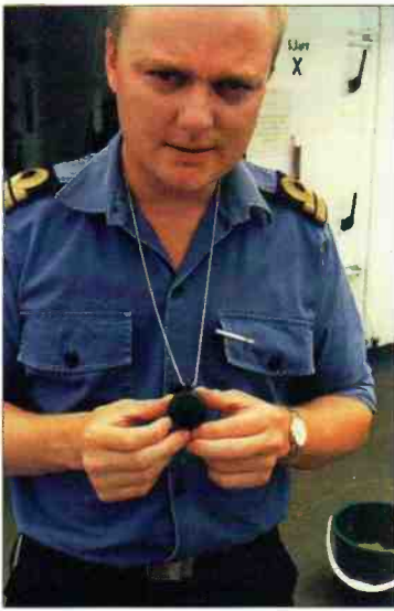
Phosphate glass dosimeters issued to Tui's crew monitor cumulative exposure to gamma radiation.
