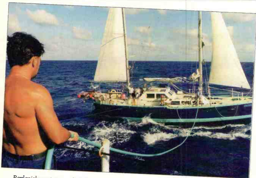
Replenishment at sea (RAS). Gemini Galaxsea receives supplies of fresh water and diesel from HMNZS Tui.
