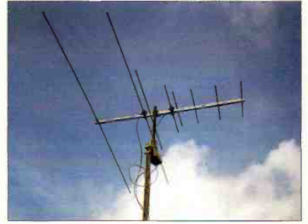
Shaun Taylor's compact all-channel v.h.f. antenna, mounted on a rotator.
