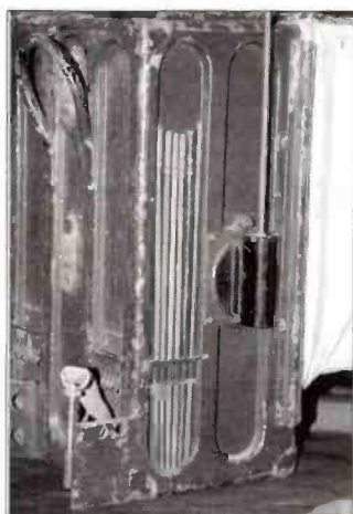
Fig. 7: Side of WS 18 showing antenna rods.
