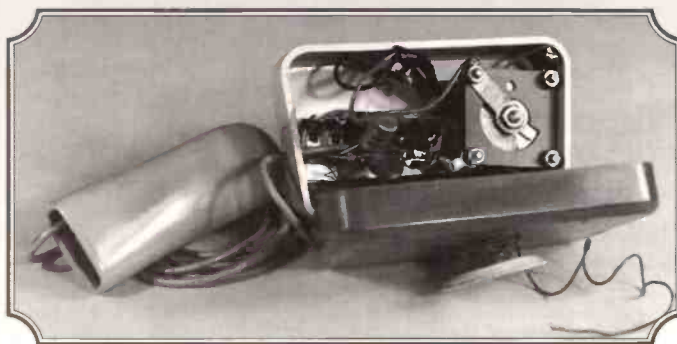
The inside of the Dewtron Wave Trap - it is possible to fit a PP3 battery in here too! The sucker on the back is clearly visible.
