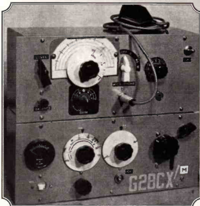
Fig. 1: Complete top-band transmitter/receiver designed and operated by the author circa 1954/5.
