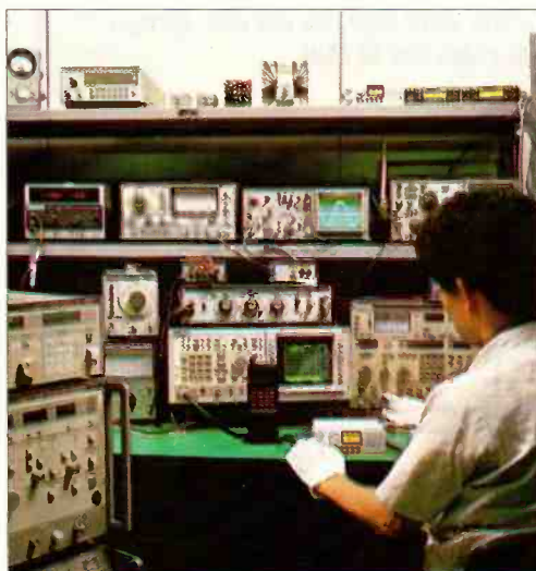
Final quality checks on an MVT-8000.
