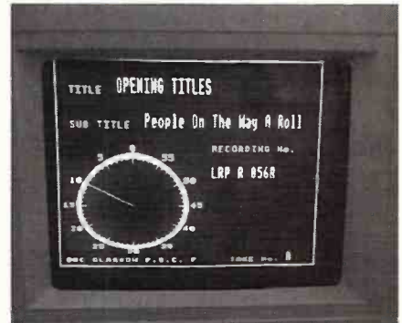
Fig. 3: John Locker snapped this VTR clock ex BBC Glasgow en route via 13°E to TV Centre, London. This heads the 'A' roll suggesting that there are additional inserts on another tape being called 'B' roll, etc.
